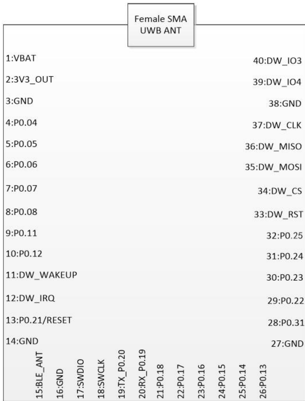
Figure 6-1: SKU620Module Pinout (TOP View)
