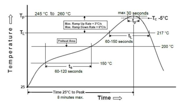
Figure 6: SKG10B Typical Leadfree Soldering Profile
