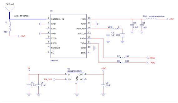
Figure 7: SKG10B Typical Reference design schematic
