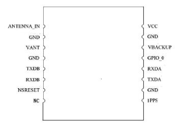
Figure 2: SKG10B Pin Package
