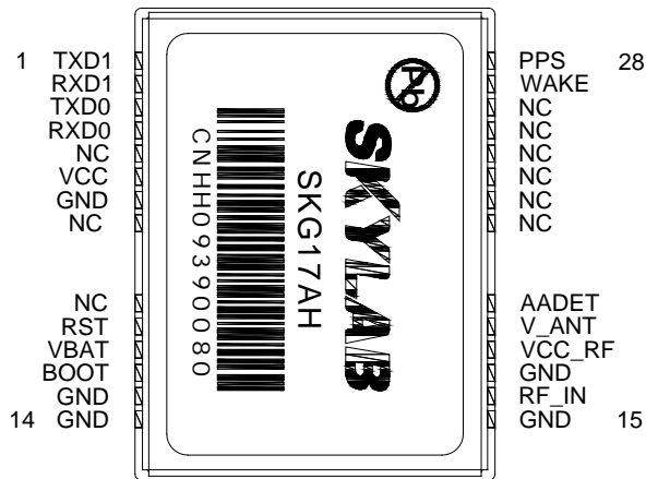
Figure 3: SKG17AH Pin Package
